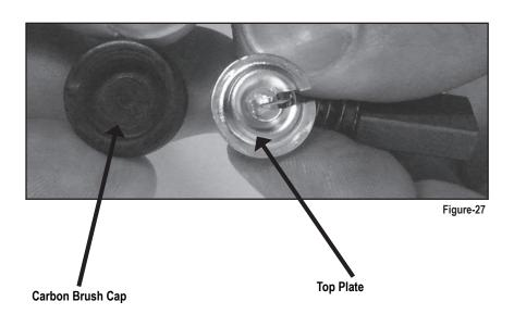
7. Check to see if the two parts move freely by pushing the top plate of the carbon brush into the recess on the bottom of the carbon brush cap and rotate.
