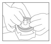
ADAPTER RING - For use on BEARING HOUSINGS (2) less than 2.5"
