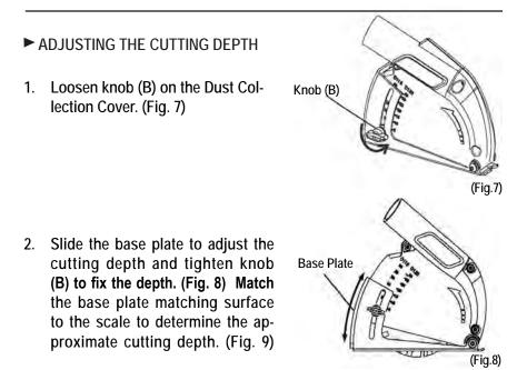
Use D115 scale for 4.5" (115mm) diameter blade and D125 scale for 5" (125mm) diameter blade. Cutting depth is indicated by millimeter.
