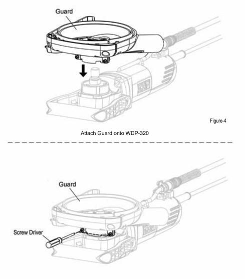
Fix two screws of the connector using a screw driver
