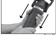
NOTE: Do not twist case in a side to side motion when pulling back.
