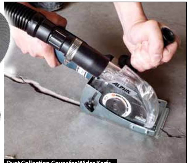
Dust Collection Cover for Wider Kerfs ECOGUARD TYPE W5
