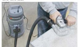
**ECOGRINDER:** Watch the Alpha® Ecogrinder in action, a high-performance grinder with a built-in vacuum system...virtually dust-free grinding solution!
