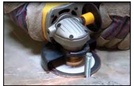
Hybrid Blade for Intricate and Flush Cutting Applications
