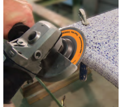
VEXCEL RIGID DISC (Stone Grinding)
