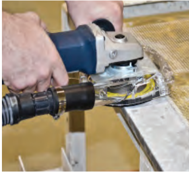
ECOGUARD TYPE G + SPIKE DISC (Mesh Removal)
