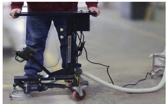
ECOGRINDER + CADDY (Surface Preparation)
