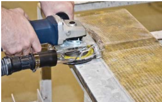
ECOGUARD TYPE G + SPIKE DISC (Mesh Removal)
