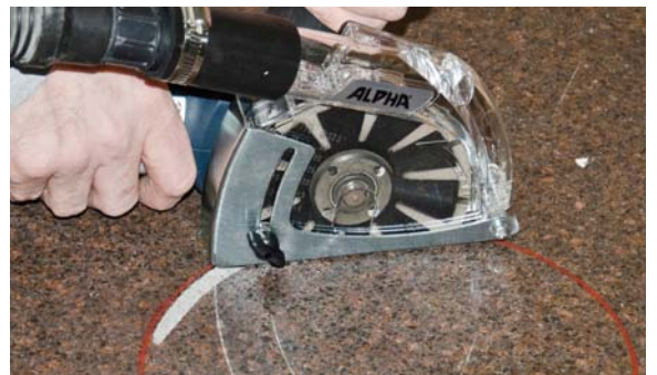
ECOGUARD TYPE W + CONTOUR BLADE (Curve Cutting)
