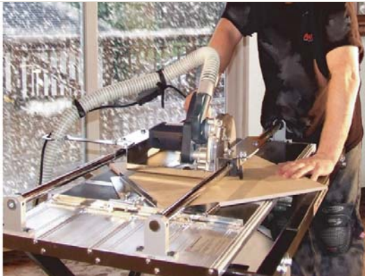
Ecocutter Dry Tile Cutting System
