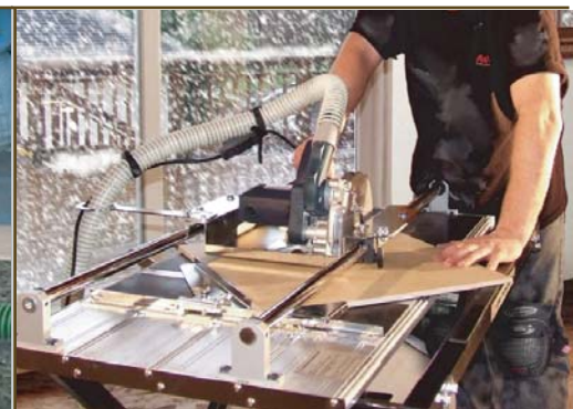
Ecocutter Dry Tile Cutting System
