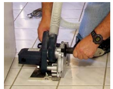
Hot-Rod Blade for Grout Removal
