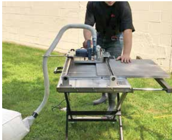
DRY PORCELAIN PAVER TILE CUTTING SYSTEM PORTABLE CUTTING SYSTEM
