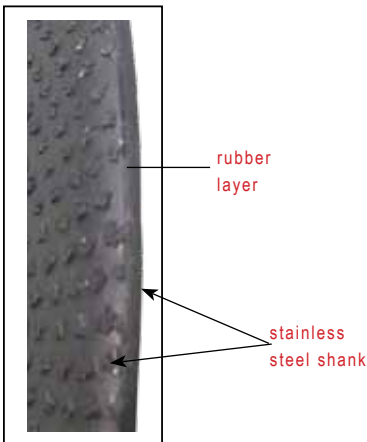
flexible sandwich construction
