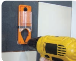
Place tip of drill bit into the guide position. Then start drilling.
