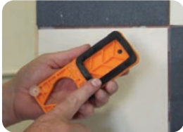
Soak the foam rubber on the back side with water.
