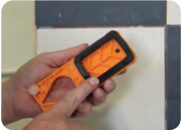
Soak the foam rubber on the back side with water.
