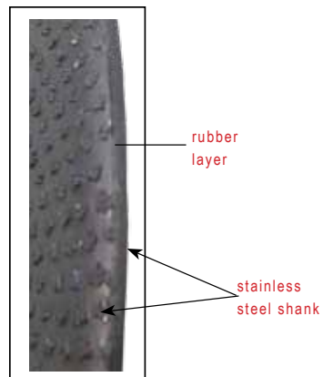
flexible sandwich construction
