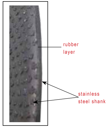
flexible sandwich construction
