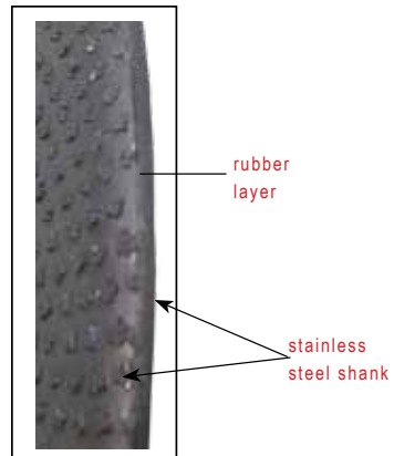
flexible sandwich construction
