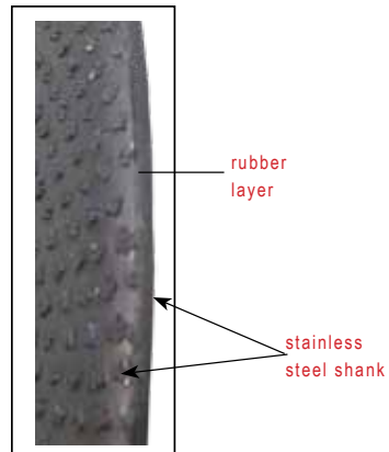
flexible sandwich construction
