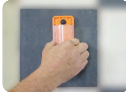
Press the body to the tile and make sure it adheres properly.
