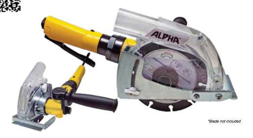
This system is recommended for virtually dust-free masonry cutting applications using a diamond blade. It fits not only standard cutting blades but also wide kerf blades for tuck pointing, crack chasing and grout removal. Also, great for curve cutting blades for sinkhole cut out applications. To keep the keep dust to a minimum, an optional water feed system is available.
