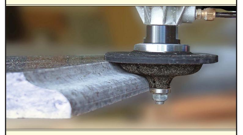
Alpha® introduces a new addition to the Profiler Series with the Profiler F, commonly known as Ogee. Since creating an Ogee edge requires a large amount of material to be removed, Alpha® recommends a two-step process to make your
