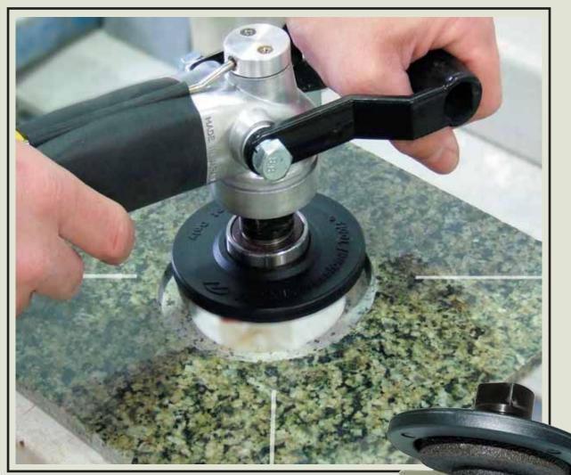
Be the first in your field to take advantage of a new and unique product developed exclusively by Alpha Professional Tools® for creating edges for recessed drains. Introducing the Alpha® Profiler Q-Series. Designed to create a 90 degree edge to accept recessed drains. Like all other Alpha® Profilers, the Profiler Q-Series is easy to use and fits on most water-fed polishers and grinders.
