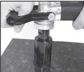
C-Shaped Handle during Drilling Application
